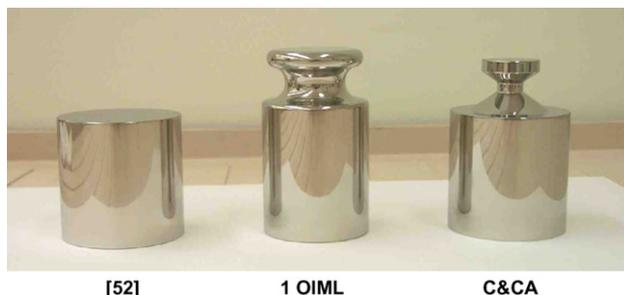
**Figure 1.** Transfer Standards. The control standards are visually indistinguishable from the transfer standards.
